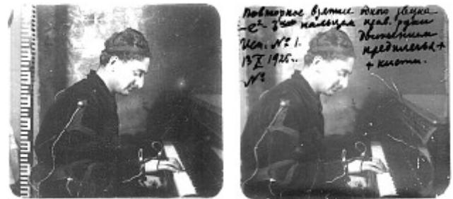
Fig. 1 Cyclogram of the piano touch measurements at GIMN, Moscow 1925. Loops above the hands of wired up pianist trajectories of lamps on his hands, printed on the photo plate. It is a stereo photograph to get the spatial information about trajectories.
