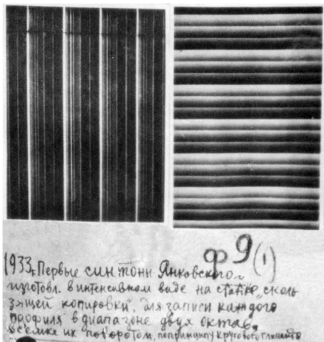
Figure 6: Variable density images of the waveforms, produced by Boris Yankovsky in the middle 1930s. Andrey Smirnov archive.
